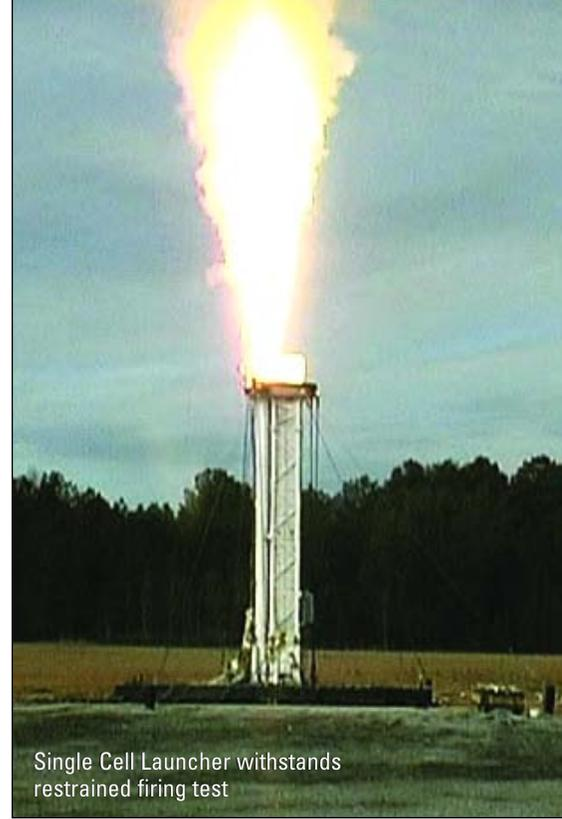
Single Cell Launcher withstands restrained firing test
