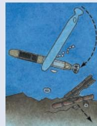
The SUBMATT® sinks away from the submarine ensuring separation prior to motor startup.
