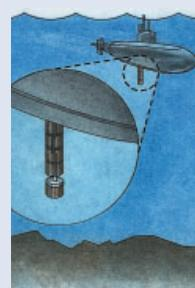
The submarine crew loads the SUBMATT®/ TDULK into the TDU and deploys it on command while underway and submerged. TDULK allows the SUBMATT® to exit freely from the submarine without damage.
