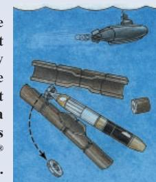
TDULK and the SUBMATT® target sink safely away from the sub, the protective sabot separates and a launch weight falls from SUBMATT® as it rotates.
